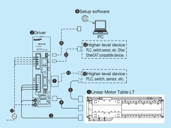
Example of system configuration for twin table
