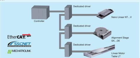
Remark: Please also note that the driver (MR-J4-10B made by Mitsubishi Electric Corporation) compatible with SSCNET II/H and that compatible with MECHATROLINK ( $\Sigma$ -7 Series AC servo amplifier made by Yaskawa Electric Corporation) will be prepared based on usage. If needed, please contact IKO.
