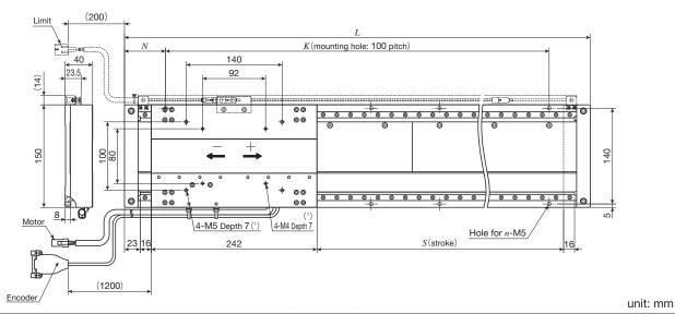
Mounting holes of bed Overall length Total mass of table Mass of moving table Stroke length Identification number Lkg kg N K LT150CEGS- 400 400 720 600 14 12.4 60 LT150CEGS- 600 600 920 800 15.5 60 18 LT150CEGS- 800 800 1 120 1 000 18.6 60 22 1.5 LT150CEGS-1000 1 000 1 320 60 1 200 26 21.6 LT150CEGS-1200 1 200 1 520 60 1 400 30 24.7
