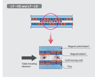
By switching the coil current to certain direction corresponding to the flux direction, continuous thrust force in a certain direction can be obtained and linear motions of the rotator is maintained. In the High Thrust Series, as the coils are densely arranged in vertical magnetic flux generated by a pair of coil yokes arranged one above the other, it can produce extremely high thrust force although it is small.
