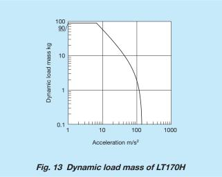
Remark: These are values calculated based on the thrust force with table moving speed set to 1,000mm/s.
