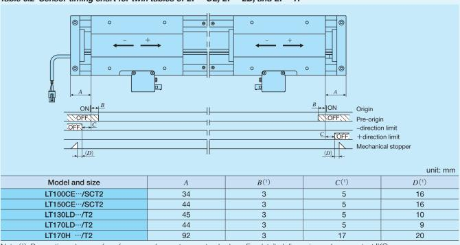
Note (1) Respective values are for reference and are not guaranteed values. For detailed dimensions, please contact IKO. Remark: For the specifications of respective sensors, please see the section of sensor specification in General Explanation.
