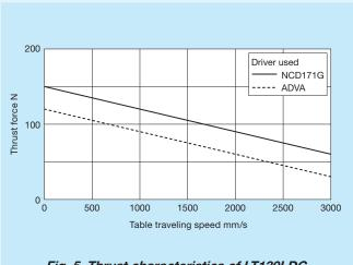
Fig. 5 Thrust characteristics of LT130LDG
