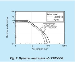
Remark: These are values calculated based on the thrust force with table moving speed set to 1,000mm/s.
