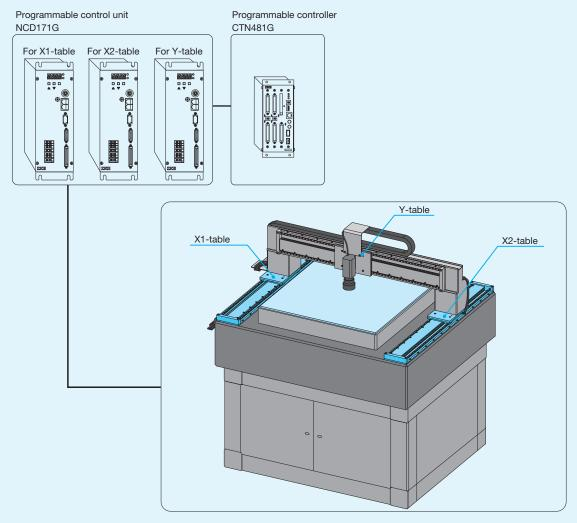
This configuration example is a system configuration of parallel operation of X1 and X2 tables with IKO programmable controller CTN481G set as an upper controller.
