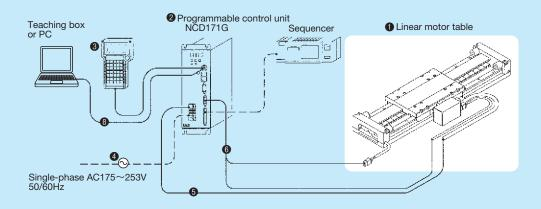
• Example of system configuration for twin table
