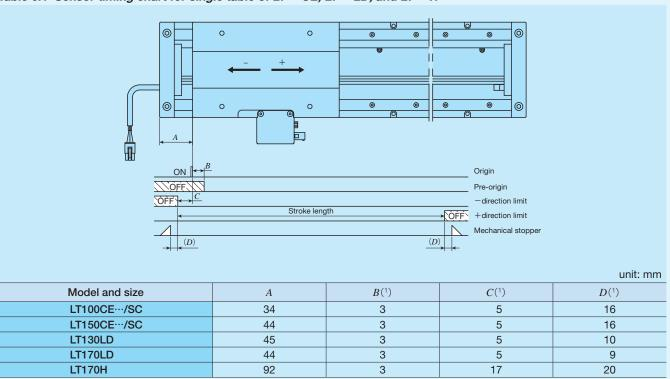
Note (1) Respective values are for reference and are not guaranteed values. For detailed dimensions, please contact IKO. Remark: For the specifications of respective sensors, please see the section of sensor specification in General Explanation.
